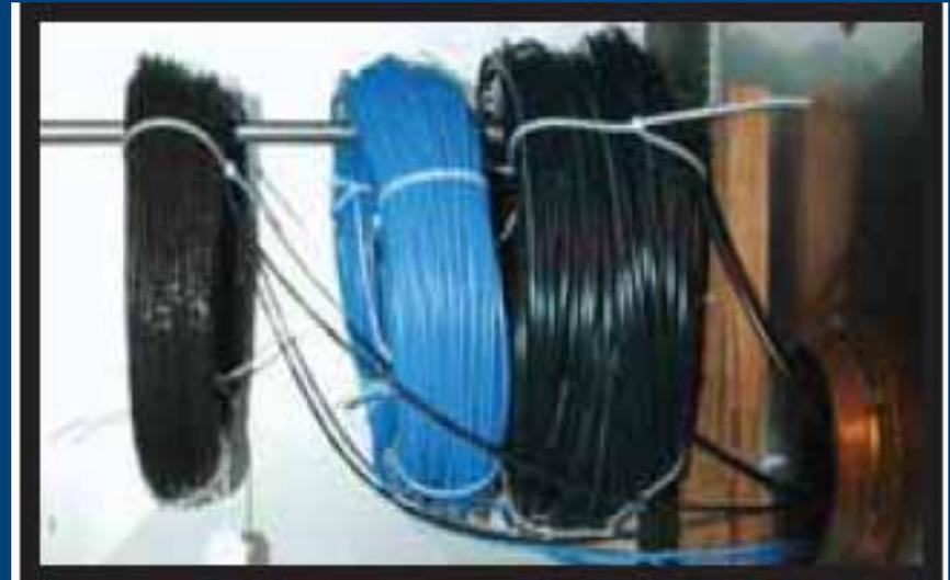
The cables were tested, as suspended, in a high temp oven.
