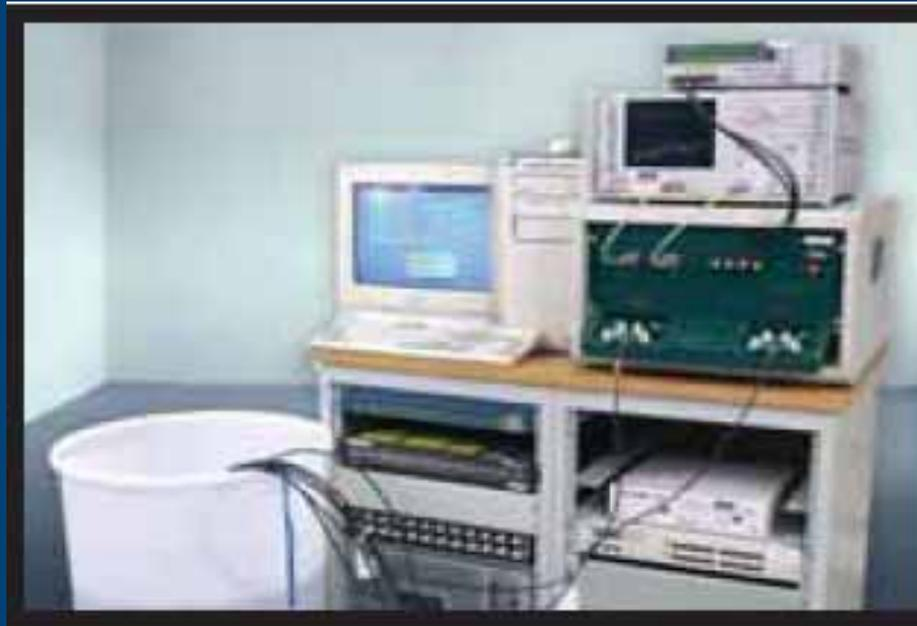
**The water bath test is a six-month long test, with the cables fully submerged in water.**
