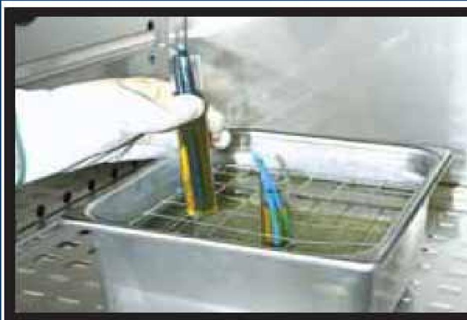
**The oil bath test, conducted as specified in UL 1277.**
